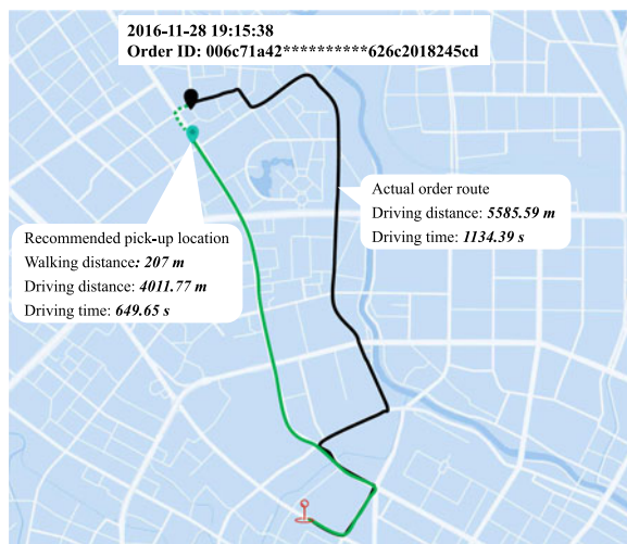
Fig. 12. A concrete example of pick-up location recommendation that performs better than the actual order route on driving distance and time.
