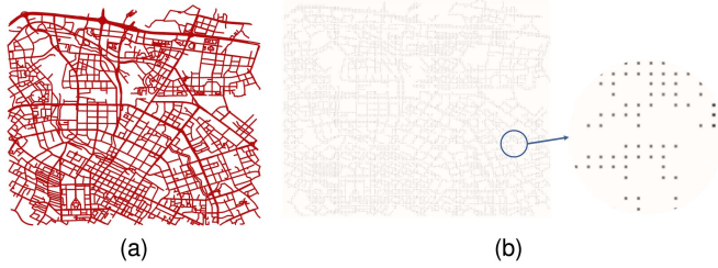
Fig. 6. (a) An example road map matrix after QGIS processing; (b) the pruned action matrix by applying the filter mask.
