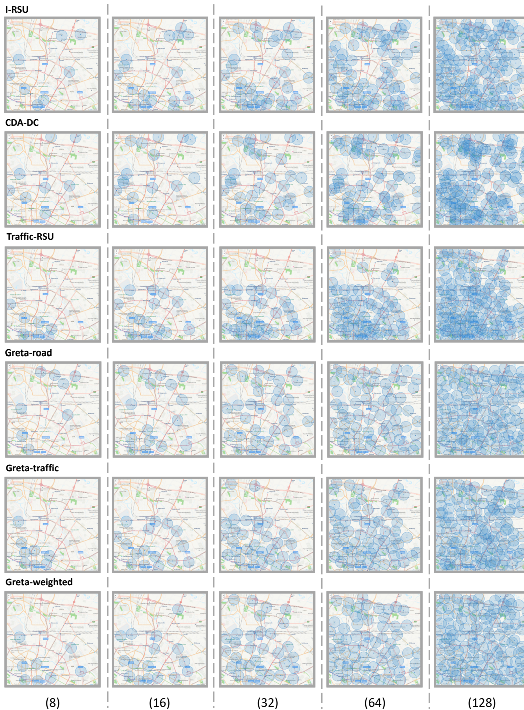
Fig. 7. Comparisons on the RSU deployment plans of different methods with different available numbers of RSUs, i.e., N = 8, 16, 32, 64, 128 . The upper three rows visualize the deployment results of three baselines, respectively, and the lower three rows show the results of Greta's variants that aim to optimize road coverage, traffic coverage, and the weighted combination of road and traffic coverage, respectively.
